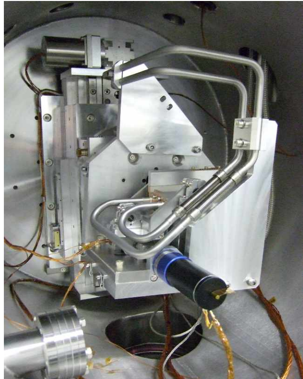
Fig 3: The in-vacuum mechanics incl. water-cooling
