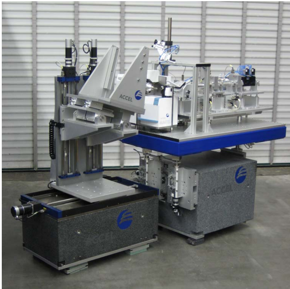
Complete endstation for Protein Crystallography as installed at BESSY
